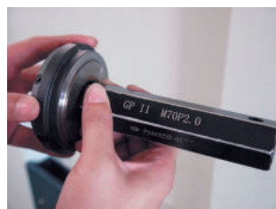
Check the thread precision by a gauge to ensure ISO 4H
