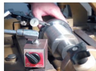
Measure the thread run-out a gauge to ensure ISO 4H
